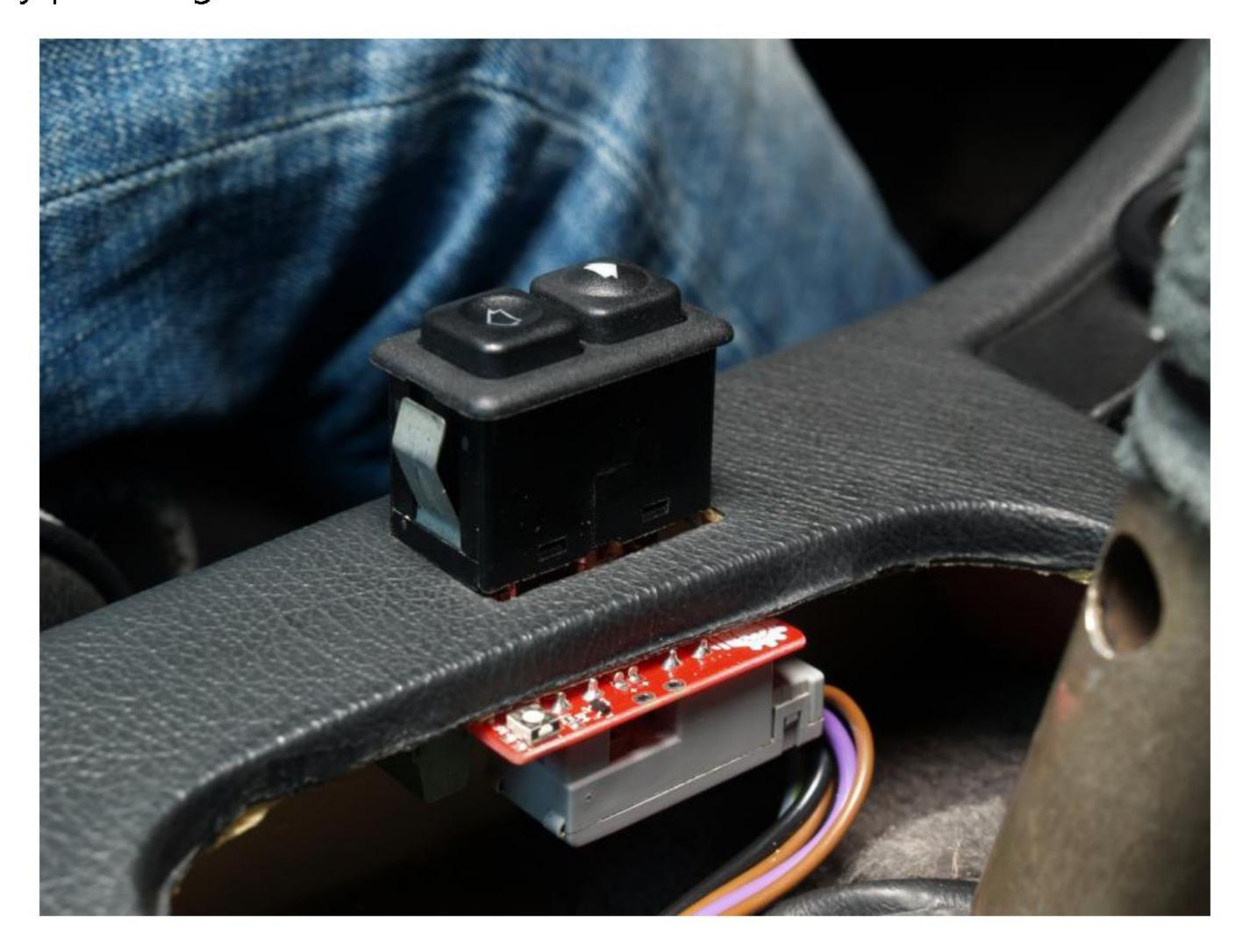
f. Push the switch through the hole so it sits firmly in its place. You might have to move the wiring a little to make room for the switch to sit properly.
