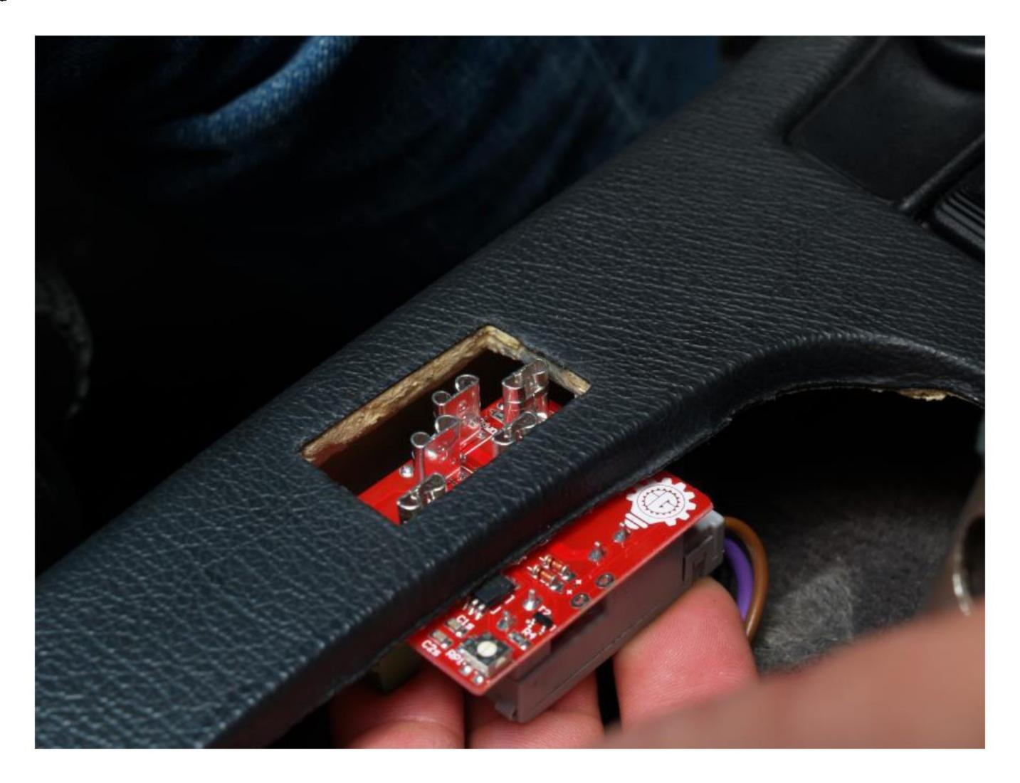
d. Take the window switch and from the top side of the hole align the pins to the fastons on the module through the hole.
